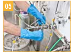
05 Connect to the cleaning ring
