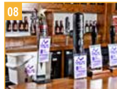
08 Place CIP tags on taps to show clean in progress
