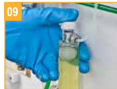
09 Bleed fobs until full of cleaning solution
