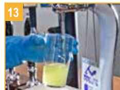
13 Pull off 1 pint of fluid per line
